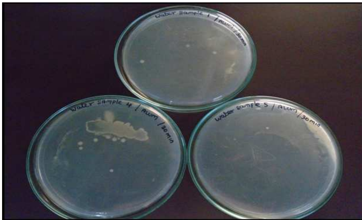
Figure No.8: Water samples treated with alum
