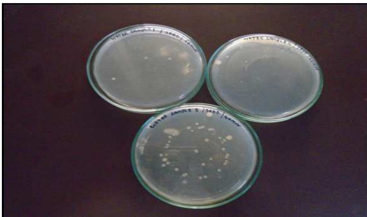
Figure No.7: Water samples treated with S.potatorum seed powder
